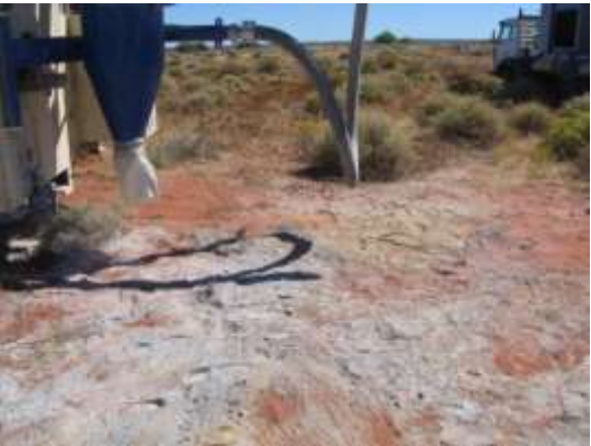
Photo E-3: Localised drilling dust and dust bagger
